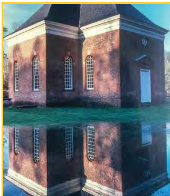
REFLECTING WATER Taken in March 1989, this stunning photograph reveals how rain water accumulates in the church yard and fails to drain away. Capturing and diverting this water from the church is the primary objective of the rising damp mitigation project.
